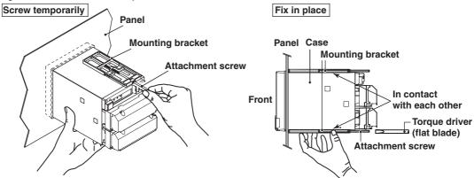
(The figure shows the DX100P when the mounting brackets are used on the top and bottom of the case.)
